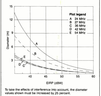
Even though the CNR at impulse noise threshold for programming material is about 10 dB, a CNR of 12 dB will ensure additional margin for rain fades as well as allow impulse-free reception of highly saturated hues, as in color bars. Figures 2 through 5 show the diameters required to satisfy both the CNR and SNR constraints for NTSC, ACTV broadcast standard (same as for NTSC), ACTV production standard, HDS-NA for 25 percent
