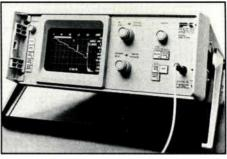
The OTDR gives a ''picture'' of the fiber along its length.
