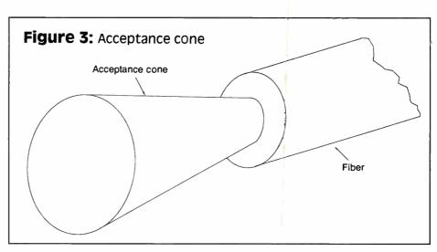
is 125 or 140  $\mu$ m. Multimode fibers allow multiple modes (light rays) to enter and travel through the core. Single-mode fibers have core sizes of 8.3, 8.7 and 9  $\mu$ m. Cladding diameter is 125  $\mu$ m. Singlemode fibers allow only one mode to enter and travel through the core.
