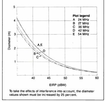
parametric values are appropriate for use in the link equation defined in last month's installment as Equation 1:
