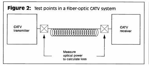
installation crew and go fix it. If a splice or connector with poor optical return loss is spotted, it needs resplicing or cleaning and reconnecting with new index matching jell to get rid of the back reflection that is bothering the laser transmitter.
