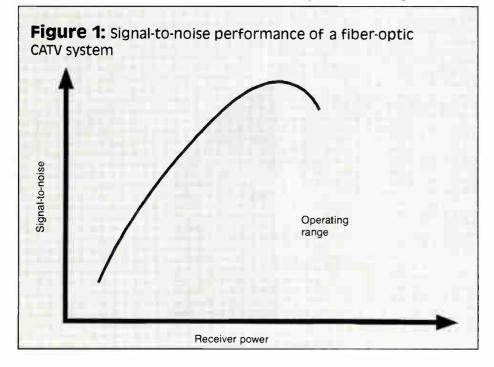
"The secret to good performance is exactly the same as with a purely electrical system: maintaining an adequate signal-tonoise ratio."
