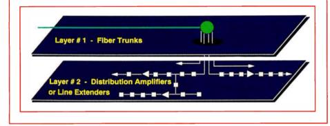
rules of designing cable plant are evolving and we need to rethink how we do these things. Fiber has very low loss, so let's use it for trunks and keep the coax for the feeder where it is very cost-effective. In most cases the cable is already in place, so we can use that for the last mile to the home.
