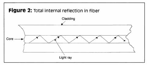
within an area outside the fiber known as the acceptance cone (Figure 3) will enter the core and be reflected down the fiber; all other light will be lost. The acceptance cone area is defined by the quantity called *numerical aperture* (NA), which is a measure of the light gathering ability of an optical fiber.
