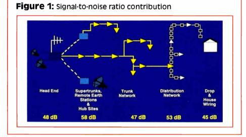
Figure 2: Conventional coax plant architecture
