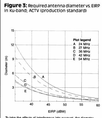
To take the effects of interference into account, the diameter values shown must be increased by 25 percent.
