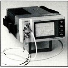
The optical fault finder is a low-cost alternative to the OTDR to find cable faults.
