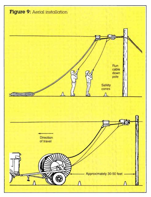
come. The usual problems with aerial lines are caused by ice and wind, and the danger of falling trees, runaway cars and bullets. With fiber you have the added concern of extreme temperature variations in harsh environments and the danger of ice forming and crushing the cable. I don't recommend aerial cable installation unless there is absolutely no other alternative.
