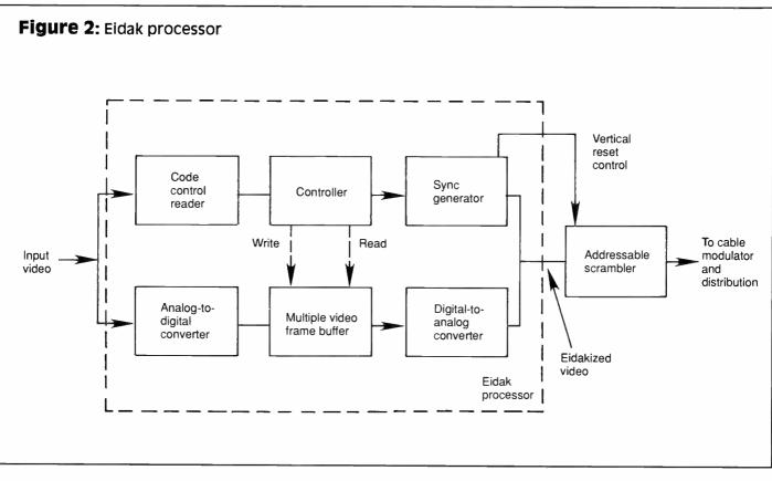
sync, some resynchronization must be provided for cable scramblers, which typically are dependent on precise VBI timing. For remote hub operations of scramblers, frame length data is encoded into the VBI and at the hub location an Eidak scrambler interface (ESI) converts the frame length information into resynchronization signals for the scrambler.
