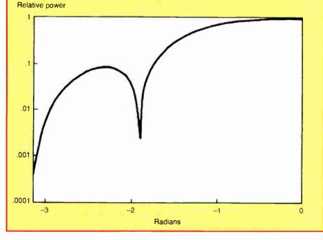
Stagger stacking may create more harm than good if the interfering signal arrives from a relative angle less than 172° or more than 188°. It is instructive to follow the development of the radiation pattern backlobes on Figures 4 through 6.
