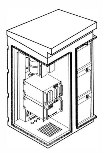
Separate Fully Accessible Battery Compartment
