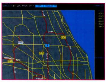
Three levels of map displays can be viewed on the dispatcher's screen. The maximum view is 24x16 miles (above), the minimum is 6x4 miles (below).
