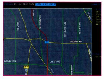
To assist dispatching, the operator can display the five closest vehicles to any street intersection, site or Tracknet-equipped unit stored in the computer's data base. This display can be increased to the closest 12 units with a single key stroke. The tabular display contains driving distances, listing units in ascending order (i.e., the closest one first). Under the map display the reference point (color-coded blue) is centered on the map.
