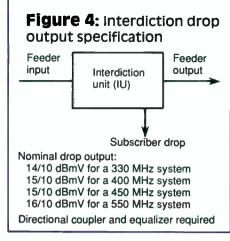
with interdiction parallels design with taps. With interdiction, the tap value is determined unit-by-unit with a plug-in directional coupler. Selection of the directional coupler is a similar process as selecting a face plate value in traditional tap systems.
