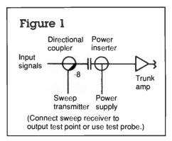
a system problem needing repair. Major response variations indicated system problems, while minor variations were compensated for using the adjustments on the amp module.
