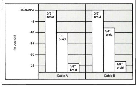
connector retention of the cable. A connector on a 53 percent braided cable should not be expected to have the same retention force as on a 95 percent braided cable. Figure 1 illustrates how the connector retention force varies with different braid coverage drop cables. These differences are mainly due the amount of metal in the outer shield.
