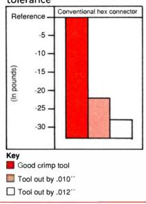
able long-term retention of the large variety of drop cables over a wide range of temperatures, wind flexure and vibrations. Close study of commonly available F-fitting components reveal thousands of possible combinations of installing a one-piece, RG-59, crimp type F-fitting onto an RG-59 drop cable. The advent of more universal sized connectors has greatly reduced the number of combinations, but selection of compatible components is still very important.
