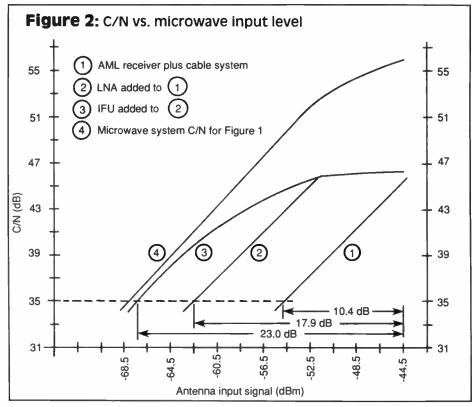
45.1 dB for 6-foot, and 41.6 dB for 4foot diameter dishes. A 2 or 3 dB field factor accounts for miscellaneous additional loss at waveguide flange interfaces and small imperfections in antenna alignment.
