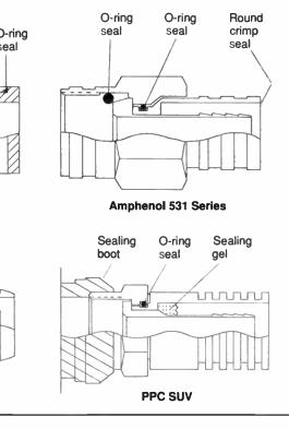
in the convenience and mechanical performance of the connector, but virtually no development on the environmental performance of the interface. It only has been in the past seven or eight years that we have seen an emphasis on developing F-connectors that seal the interface as a function of connectorization. When properly assembled, these new connectors work very well to keep moisture out of the connection. Figure 7 is a look inside some of the more common sealed F-connectors.
