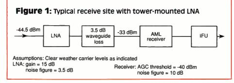
dB and the cable plant contribution is 47 dB, power addition of the two C/N ratios gives an overall 46 dB. On the other hand during a deep microwave path fade, the 35 dB of the microwave system is the dominant source of noise and the above cable plant's "last subscriber" *should* be looking at a 34.7 dB picture.
