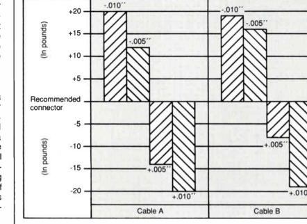
Figure 2: Cable retention with different crimp ring IDs
