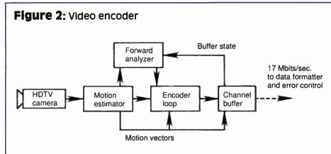
and, of course, a great deal of repetition from frame to frame, Bell Laboratories has been active in TV compression since the early '50s and in **DSC-HDTV** it uses motion compensated transform coding that exploits both the temporal and spatial redundancy in the HDTV signal.
