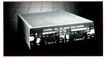
The AGC module itself is  $1.6^{\prime\prime}$  H x  $5.5^{\prime\prime}$  W x  $10.5^{\prime\prime}$  D and is designed to be mounted in Learning's PMU401 panel mount. The panel mount is  $19^{\prime\prime}$  W x  $1-3/4^{\prime\prime}$  H and will hold either three AGC modules or two modules and a PS420 power supply. Up to five AGC432s can be powered from the PS420. An external power supply also can be used; requirements are +24 volts DC @ 150 mA per module.
