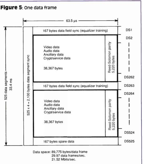
ments makes possible the reliable detection of data segment sync even under severe interference conditions such as ghosting.
