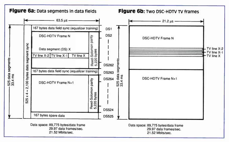
ure 6a each data segment carries the information for 3 DSC-HDTV scan lines, which when sequentially processed by the receiver decoder (see Figures 3 and 4) produces two progressively scanned DSC-HDTV frames as shown in Figure 6b.
