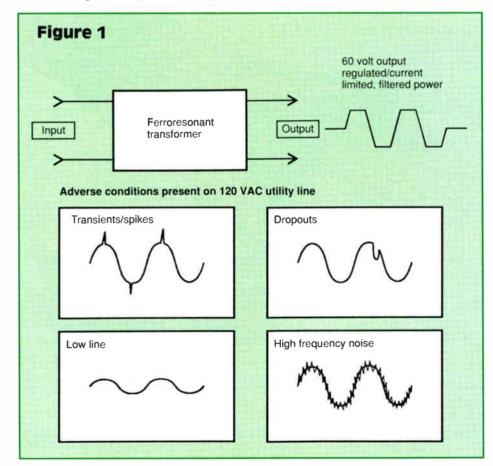
ly useful in the cable TV application because it protects the active devices from damaging voltage fluctuations; e.g., brownouts and prolonged high and low line conditions. This feature also allows reliable operation of the cable system, even if the input voltage is consistently low.
