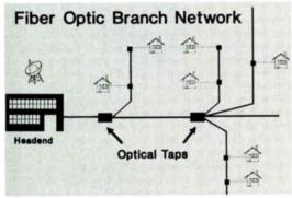
By reducing fiber counts and transmitters (lasers) with Gould Fiber Optic Splitters.
