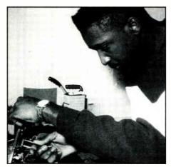
4) Converters are disassembled and any remaining paperwork filled out. From here they go to a repair staging area.
