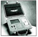
Model 1210 TDR. **Cable Fault Locator**
