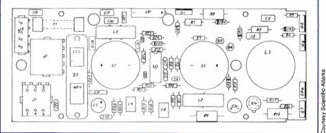
chassis. Once removed, the PC board must be mounted onto a jig that will simulate the chassis by tying these foil areas together. I use a jig made from an aluminum sheet measuring 7 1/2 inches by 3 inches, with four 1/2-inch metal spacers mounted so they are aligned with the PC board's mounting holes.
