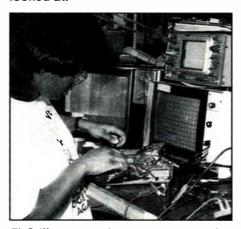
7) Still at operating temperature, the repaired converters undergo full alignment and timing adjustments.
