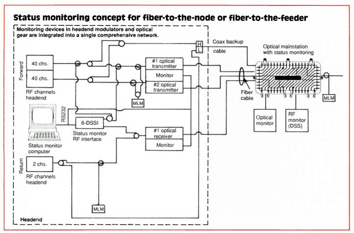
most common locations are: output of headend combiner, input to optical transmitter, output of optical node, end of trunk cascades or feeder cascades. The MLM works in any system; even one-way plant. It can either communicate using the return signal path or standard dial-up phone line.
