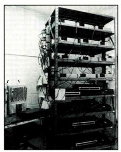
8) After alignment, all units spend a minimum of four hours at 105°F in the "burn room" while still plugged in and operating.
