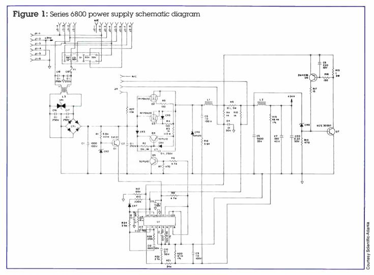
supply, which means that anything between the fuse and the crowbar are put under stress while the fuse takes time to blow. The result is that the circuitry making up the overvoltage protection often burns up, frequently making quite a mess of the board.
