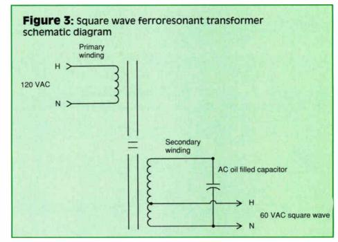
60-volt AC output: The ferroresonant transformer is the most effective and widely used design for protection from transient events; however, other devices are used in conjunction with the transformer to protect the active devices connected to the power supply
