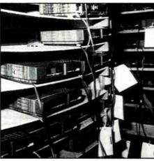
5) Before actual repair, all converters are placed on a pre-heat cart, where they have a chance to warm up for two to six hours before being looked at.
