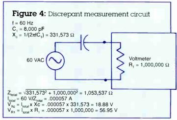
varies inversely with the frequency. This opposition is called *capacitive* reactance, and can be calculated according to the equation:
