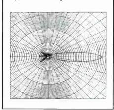
radiating elements, forming antenna arrays. Elements can be phased to give the various azimuth distributions and beam tilts below horizontal. Increasing gain is realized by stacking an increasing number of "bays" or shorter tubes.
