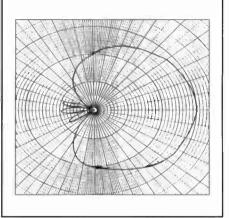
**Figure 5:** Vertical plane radiation pattern for hemisphere coverage
