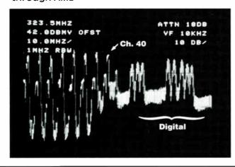
SkyPix channels can occupy in the cable system. Analog video channel assignments are placed in a data base to allow the controller software to determine optimal digital channel structuring (within available spectrum) for minimal intermodulation distortion of all carriers (both analog and digital video). This information also is required at the receiver to facilitate digital vs. analog tuning discrimination.
