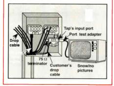
the DC that indicates the correct tap port loss. For example, a DC-24 attenuates the signal 24 dB at the tap port.
