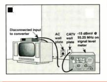
Figure 3: Checking at the wall plate with customer's TV set
