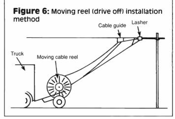
method, adequate rollers, blocks, rings or hangers must be provided to support the cable. It is recommended that a worker be placed at the cable reel trailer to prevent the reel from "hanging up" and limit tail loading of the cable during placement. Helicopters have even been used to place fiberoptic cable under some rather special circumstances.
