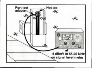
able video carrier signal level or poor picture quality at its output port indicates a defective DC.
