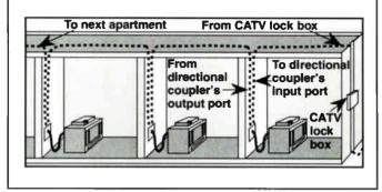
tap, or the feeder or trunk system. More than one customer will be affected. Acceptable video carrier signal level on the SLM or good picture quality on the TV test set at the tap's input port indicates a defective tap face plate. Replace the tap's face plate and recheck the picture quality.
