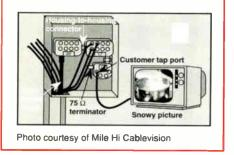
DC-30 and unacceptable signal levels or picture quality at the tap port indicate a defective DC.
