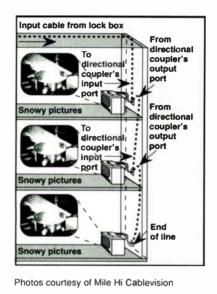
snow/no pictures on the test TV set (Figure 9) at the input to the tap indicates a defect at the tap's housing-tohousing connector, another tap, an apartment amplifier, the drop between the hot tap and the lock box, the hot Figure 16: Horizontal apartment runs
