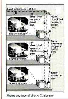
Figure 2: Measuring low video carrier signal at CATV wall plate
