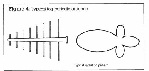
more active dipoles. Elements in front of the active dipole(s) will act as directors and those to the rear will act as reflectors. Thus the log periodic antenna will perform over a much wider band with equal gain at all frequencies. If the size of the elements changes due to icing, the active region shifts to shorter elements and the gain of the antenna does not change.
