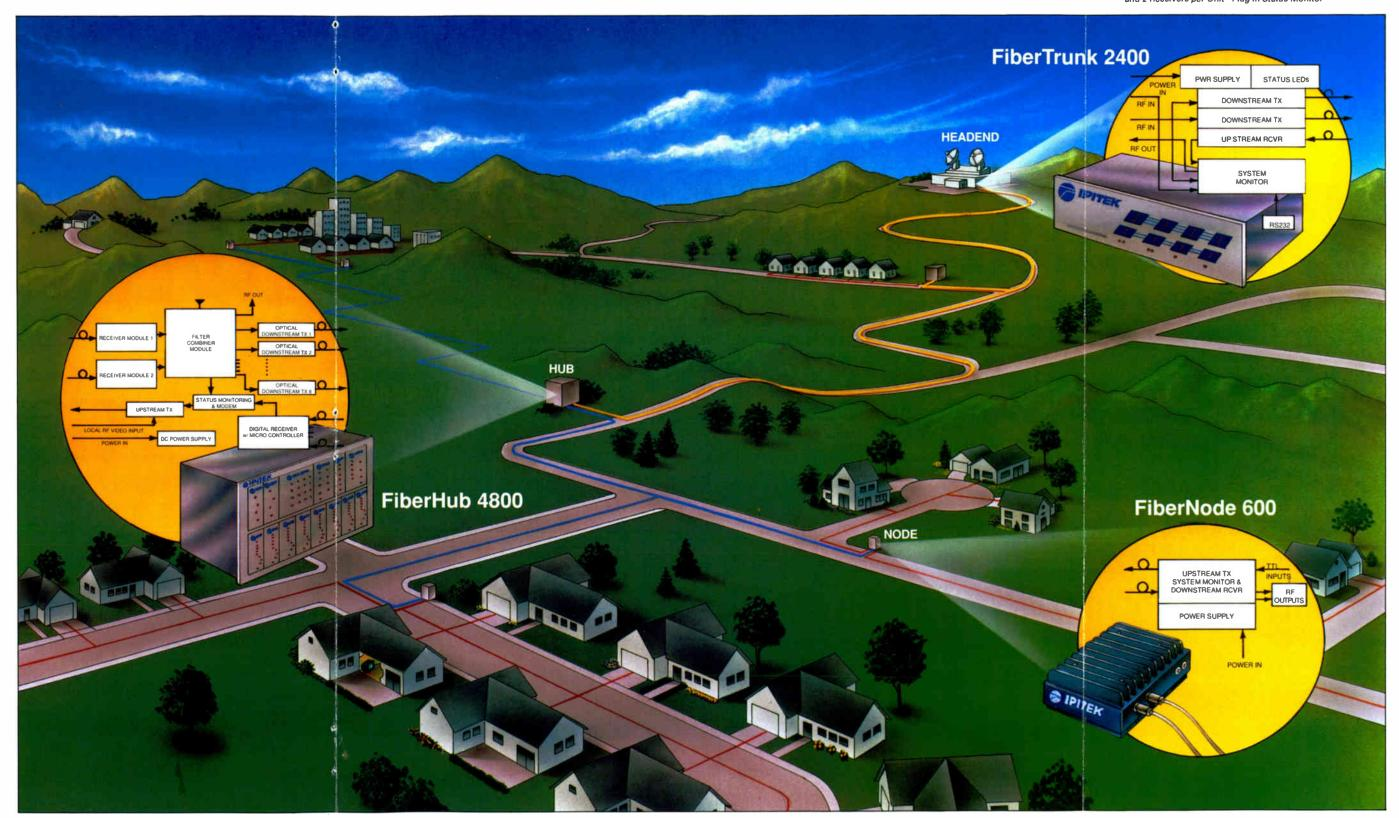
FiberHub 4800 Repeats the Optical Signal • Plug in up to 8 Transmitters • Plug in Status Monitor
