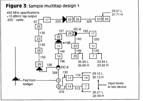
from input to tap port and includes the built-in DC value plus internal splitting (two-way, four-way, etc.). If you want a four-port 29 dB tap, you order that value!
