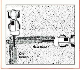
personal safety and prevent costly accidental utility line cuts. Ask homeowners for the location of all private underground electrical, phone and water sprinkler system lines. If the homeowners are not sure of the direction of the underground water lines or the underground water sprinkler maps are not accurate, dig down at the sprinkler heads to determine the direction of the underground water lines.
