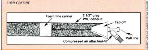
provides "a horizontal hole in the ground" for future system expansion or cable replacement. Second, it protects the coaxial cable from damage during and after installation. Third, it reduces the need for screening or for a sand cushion in rocky soil.
