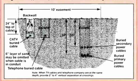
Figure 3: Typical depth of coaxial cables in a joint telephone trench
