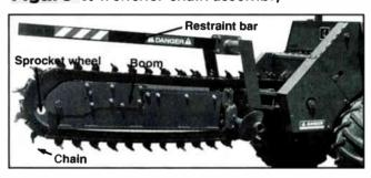
dumped against a mechanical auger, which spreads the dirt evenly on both sides of the trench or sweeps it all to one side. Chain trenchers also might have a crumbing or trench cleaner blade attached to the end of the digging chain's restraining bar. This crumbing blade is simply a small scooping blade that smooths the bottom of the trench by pulling along the loose dirt and placing it where it can be picked up by the chain.
