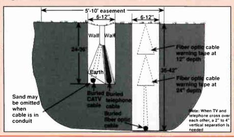
Figure 4: Typical depth of coaxial cables in a joint utilities trench
