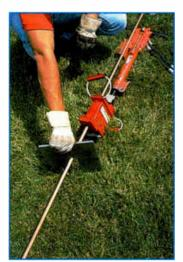
Photo 3: The release plate is positioned over the ground rod.
