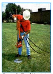
Photo 7: The Sidewinder is raised and re-attached to the rod, and the driving resumed.
