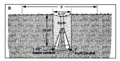
"Certain soil conditions make it necessary to backfill with a different material than was removed from the trench."
