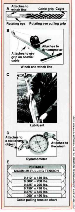
pulling coaxial cable through long and difficult conduit runs, use a dynamometer (Figure 13D) to ensure that the specified maximum pulling tension for that cable (Figure 13E) is not exceeded
