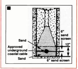
Figure 8: Unreeling coaxial cable
