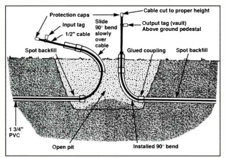
proved pulling compound, the minimum number of 90° bends, and a continuous, steady pull on the cable with no interruptions during any length of the pull. If two or more cables are to be pulled into the same conduit, pull them simultaneously and not separately. In addition, place all trunk and feeder coaxial cable in separate conduits. This provides splice-free runs and much easier pulls on long runs.
