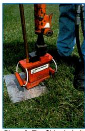
Photo 6: The Sidewinder's jaws are released from the rod.
