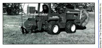
Figure 4: Feeding cable by hand
