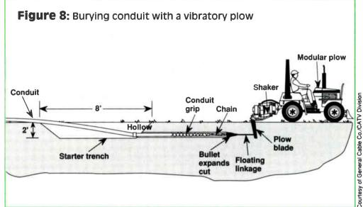
conduit to the plow blade with a pulling grip (Figure 7 on page 33); and 4) pull the conduit into the ground using the vibratory plow (Figure 8). Be sure to pull the coaxial cable into the conduit before backfilling the starter trench.
