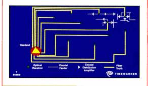
is logical to suggest that we can overcome these architectural limitations by replacing the trunk portion of the plant with low-loss optical fiber, which has the ability to provide signal transport for up to 20 miles without repeaters or amplifiers. There is indeed a different approach to architecture that meets our needs very well and, better yet, it is an architecture into which we can evolve our systems gradually from the one used at present.
