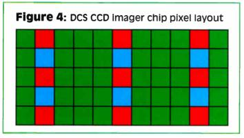
The color and monochrome backs contain the DCS's "heart": a 1,280 x 1,024 pixel imager (1.3 million pixels). Measuring 21mm x 17mm, this imager is approximately half the length and width of a 35mm film frame. Its 16 micron pixels offer excellent light sensitivity.
