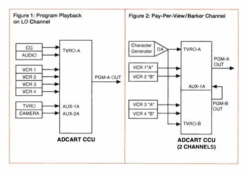
when the show absolutely must go on. As illustrated in Figure 2, the CCU's second channel can serve as a redundant "fail safe" program source. The same movie is scheduled to play on both sets of VCRs. If Adcart's automatic video quality sampling feature detects any VCR problems or any degradation of video quality, it automatically switches to the back-up source machines, unnoticed by the viewer.
