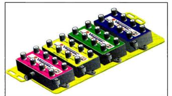
**Viewsonics** introduces a new concept in multi-output distribution taps. Using a modular concept, they developed a series of multitaps having various port values within the 16, 24, 32, and 48 port models. Home-run installs with extreme distance variations are easily served. In addition they provide for more selectivity in signal level. Tap values are from 14 to 35dB, from 5-600MHz.
