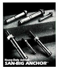
Metric Expansion Anchor • Yellow Dichromate Finish Fast, reliable, universally accepted fastening Provides high strength, vibration resistance, immediate loading capability . Two available styles: finished hex head (SB) and adjustable threaded rod (SL) . Sizes M10 (3/B")-M20(3/4") • Metric Bit included • Carries high tension / shear load and resists dynamic load conditions . Follow-up expansion ensures safety.
