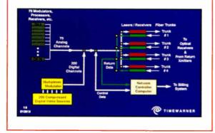
nel. Figure 11 shows that the headend for such a system will be very similar to that used in Queens, but replaces 75 of the analog video modulators with a source for 200 or more compressed digital video channels.
