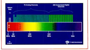
tems using the hybrid fiber/coaxial cable architecture we are demonstrating in Queens. The 50 MHz to 1 GHz spectrum is still transported on the coaxial "last mile." It contains 75 analog channels, for basic and subscription services, and 200 or more compressed digital video channels carrying HDTV and a wide array of PPV and narrowcast services. This will further increase the number of choices we offer our customers and we believe that it also will allow us to generate additional revenue.
