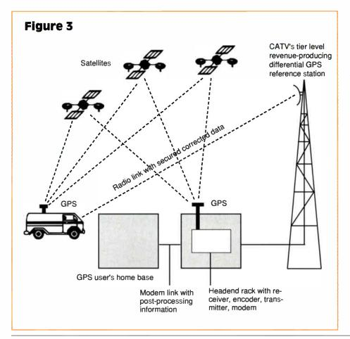
now — differential GPS (DGPS). DGPS will provide an average GPS user with 2-5 meter accuracy. Think about this for a moment — it is accuracy under 15 feet. Centimeter accuracy also is possible. This would be a topic for a whole other article.
