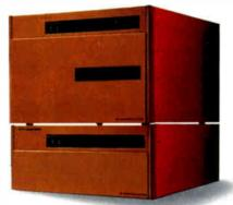
Sumitomo digital transmission equipment is cost competitive with FM. Get up to 24 video channels on a single fiber without compression or wave-division multiplexing.
