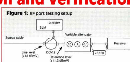
CW (carrier wave) signals differently. Run a low level (+10 to +20 dBmV) cable drop into the test area, using the best possible RF connection practices in this process of removing the possibility of leaks. Verify that the headend transmit frequency to be used for the test is the same as the equipment to be tested, since frequency errors will cause calibration errors and other problems.
