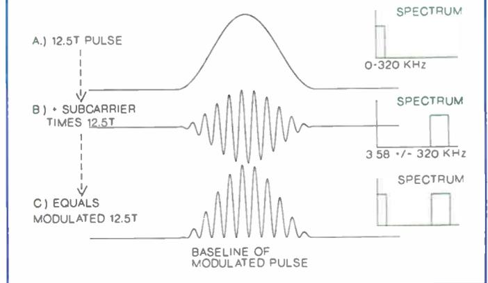
are carrying now. We call these vertical interval test signals (VITS). To evaluate the overall performance of your system, simply demodulate the output of the channels you are carrying, and look for the VITS in the VBI. You will need a waveform monitor (vectorscope required for measuring differential phase) and a good demodulator.
