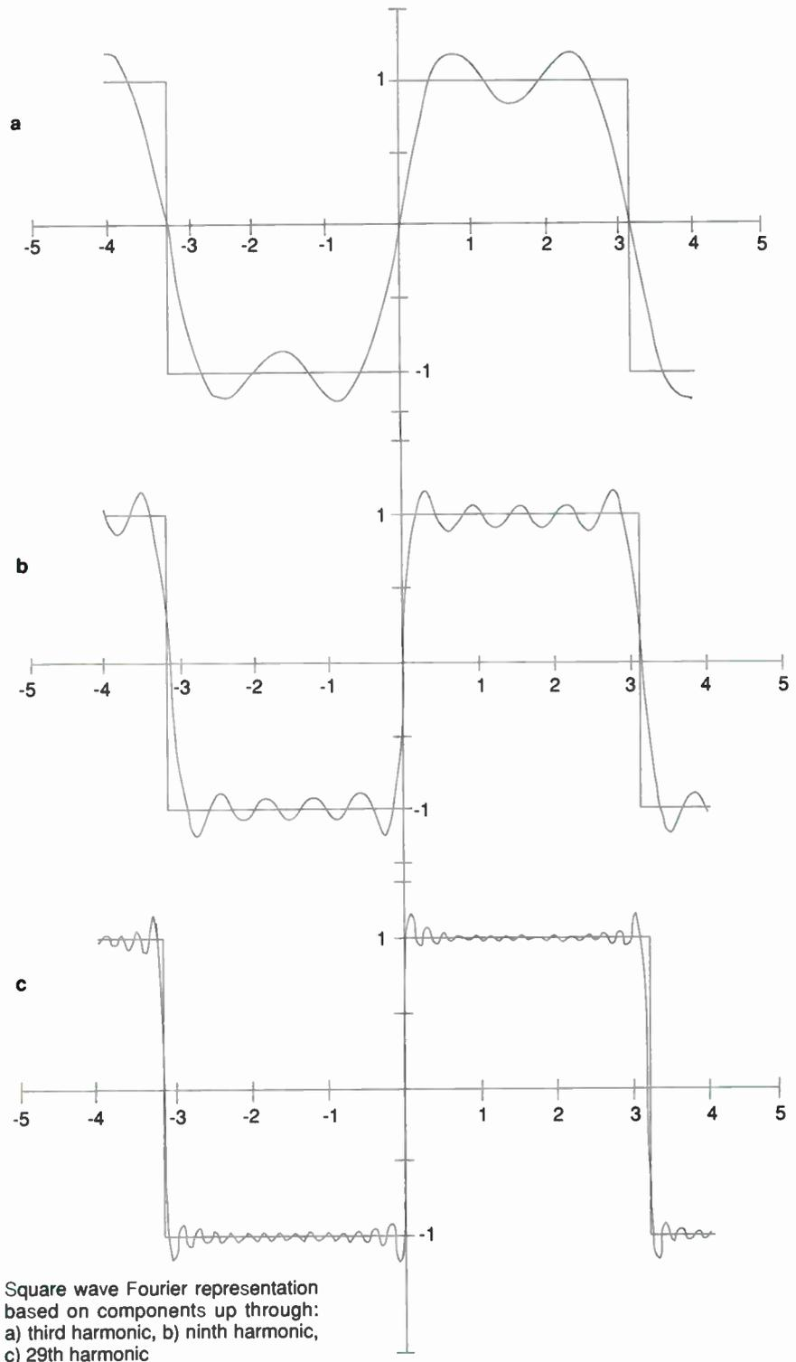
Square wave Fourier representation based on components up through:
