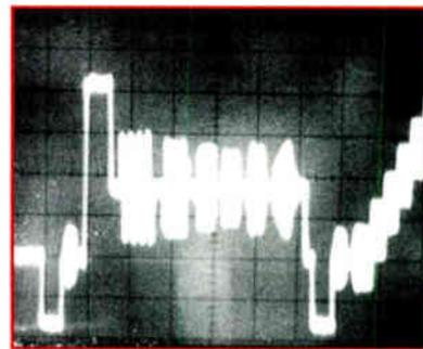
**Figure 3:** Multiburst on channel protected by positive trap
