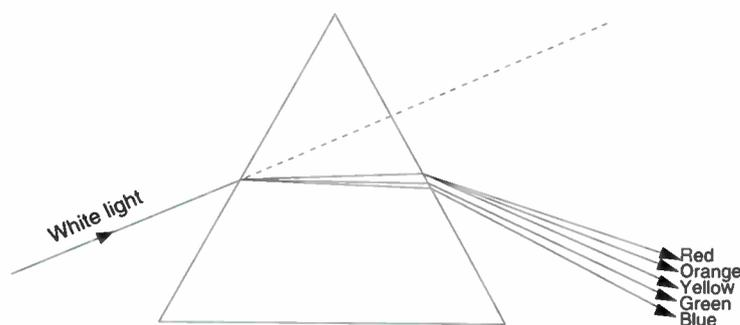
glass more than the red and therefore bent more than the red (lower frequency).
