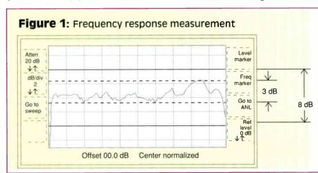
The resulting response can be displayed normalized to a selected reference location (typically the headend or first amplifier).
