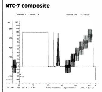
headend proof-of-performance measurements, the sin x/x test signal is ideal for measuring in-channel video frequency response of a modulator. The color bars can be used to adjust headend monitors and TV sets.
