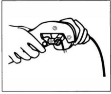
8) Put connector into correct crimp hole.
