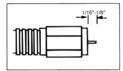
10) Check that center conductor extends out 1/16-inch beyond connector. **BTB**
