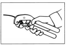
7) Put connector into correct crimp hole.
