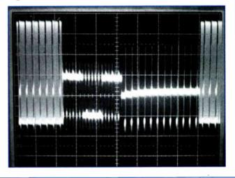
Bandwidth: 300 kHz minimum, 3 MHz preferred Frequency span: Zero span Trigger: AC line Scan time: 200 ms Video filtering: None, 1 MHz preferred
