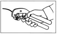
7) Put connector into correct crimp hole and squeeze until crimpers stop. Never double crimp.
