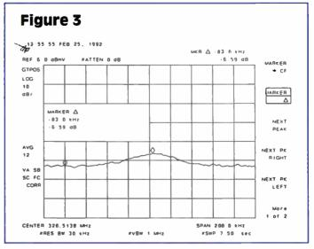
An analyzer measures in the units of dBmV for a large dynamic range. After doing some algebra one can calculate:
