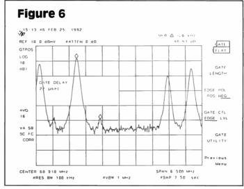
on. This is a third order distortion measurement of (visual - color + aural) carriers at +920 kHz relative to visual carrier. Also, one can see a -920 kHz product relative to the visual carrier due to (visual + color - aural).
