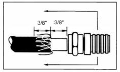
3) Fold all braid back over jacket. Make sure the foil is not torn or pushed off the dielectric.
