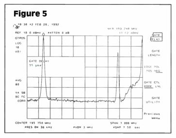
distortion product from Ch. 4 falling into Ch. 3. Two times the visual carrier of Ch. 4 minus the audio carrier of Ch. 4 creates a distortion product 4.5 MHz below the visual carrier of Ch. 4, which is 1.5 MHz above the visual carrier of Ch. 3. This is within the AML specification, but monitoring this intermod in zero span will allow the AML bias to be adjusted to minimize this intermod further. Also, observe the noise floor slope. This could be improved with an AML slope adjustment.
