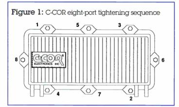
2) Close the cover until it is flush with the rubber gasket. Refer to Figures 1 and 2 for the tightening sequence for four- and eight-port housings. Thread all cover bolts finger tight to hold the cover in place. Ensure that it seats evenly on the rubber gasket.
