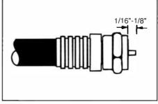
8) Check that center conductor extends out 1/16-inch beyond connector.
