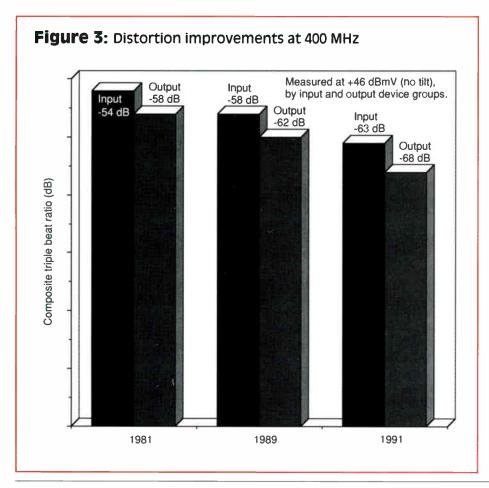
provement in composite triple beat while operated at the same level, then depending on the additional channel loading, the slightly lowered input level allowed could be considered the increase in output we didn't need. In other words, we derated the trunk by lowering the noise figure. Although this may be rarely possible, it is a card to kept in your pocket.
