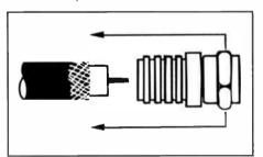
6) Push connector on to cable leaving braid folded back under crimp ring. Make sure dielectric is flush with inside bottom of connector.
