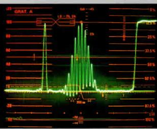
Chrominance-to-luminance delay inequality causes the 12.5T pulse baseline to have a sine wave shape. After normalizing the pulse amplitude to 100 IRE, the sine wave excursions can be converted to delay in nanoseconds using the accompanying nomograph (right). Chrominance-to-luminance delay inequality results in color smearing (sometimes called the "funny paper effect").
