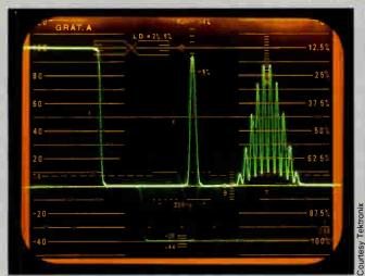
Chrominance-to-luminance gain inequality causes the baseline of the 12.5T pulse to have a concave or convex shape. It is expressed in IRE, percent or dB (after normalizing the pulse amplitude to 100 IRE). Chrominance-to-luminance gain inequality causes incorrect color saturation in the picture.
