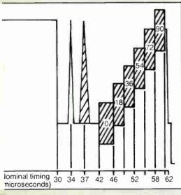
00 IRE white reference (bar), 2T pulse, lulated staircase. The 100 IRE white referting video levels, and also for measure-ind line time distortions. The 2T pulse also of short time distortion (pulse-to-bar ratio ements). The 12.5T pulse is used to deter-luminance gain and delay, and the moduntial gain and phase.
