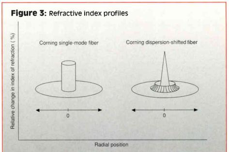
the fiber core. (See Figure 3.) The refractive index profile represents the change in refractive index of the core glass relative to the cladding glass, and typically defines the fiber's transmission characteristics.
