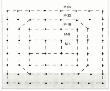
ture amplitude modulation (QAM). QAM signal waveforms are a form of combined amplitude and phase modulation. Several different constellation diagrams for QAM are illustrated in Figure 7 for M = 4, 8, 16, 32 and 64. We observe that the QAM signal waveforms result in rectangular signal space constellations when the amplitude values on the two quadrature carriers are equal.
