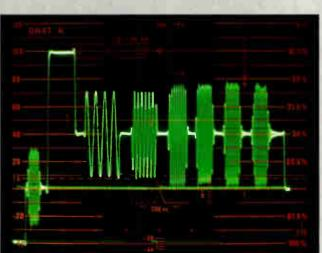
Gain-frequency distortion is a degradation of video frequency response, and can be seen as a variation in a multiburst signal's ideally flat packet amplitudes. It is expressed in dB, percent or IRE units relative to either the 100 IRE bar or some low frequency such as the 0.5 MHz packet. Gain-frequency distortion can cause other video distortions such as short, line, field and long time distortions and their visible effects in the picture.
