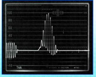
A sinusoidal distortion in the base of the 12.5T mod pulse indicates chrominance-to-luminance delay. In this example chrominance is delayed by approximately 250 ns. council hires a contractor to do a performance audit of your cable system. Which four channels do you think the contractor will select for measurement? The same four "golden" channels you selected? Not likely.
