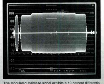
This modulated staircase signal exhibits a 10 percent differential gain error.
