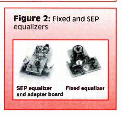
equalizers for use in Jerrold "SJ" Series trunk amplifiers. Until this year, only the variable trunk "SEP" style existed. Figure 2 shows the newer fixed equalizer and adapter board combination, and the
