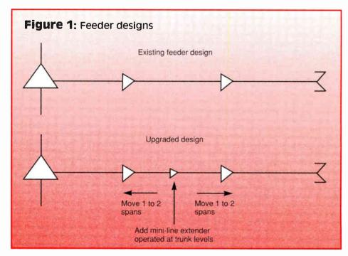
lution is the mini-LE. Figure 1 illustrates a feeder design concept involving minimal resplicing to incorporate a mini-LE that serves to more evenly distribute the required gain.
