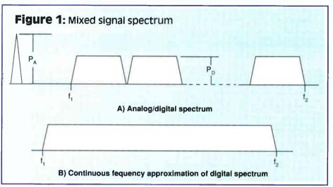
Since multiplication in the time domain is equivalent to convolution in the frequency domain, the spectrum of the distorted output may be obtained by convolution of the input signal with itself. This yields the following equation:
