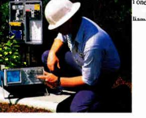
(ABOVE) THE 2714 CABLE TV SPECTRUM ANALYZER AUTOMATES ALL COMMON CABLE SYSTEM SPECTRAL MEASUREMENTS, INCLUDING THE FCC RF PROOF-OF-PERFORMANCE REQUIREMENTS.
