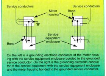
grounding, or use a special meter pan bonding connector (such as the Sachs SC51), and if the supplying electric utility does not object.
