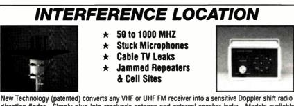
New Technology (patented) converts any VHF or UHF FM receiver into a sensitive Doppler shift radio direction finder. Simply plug into receiver's antenna and external speaker jacks. Models available with computer interface, synthesized speech, fixed site or mobile - 50 MHz to 1 GHz. Call or write for details.
