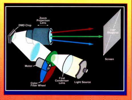
255/256ths of the frame time, 254/256ths of the frame, ..., 1/256ths of the frame time or none of the frame time. The integration of these temporally encoded brightness levels into a grey level at each pixel takes place in the eye of the viewer. In this way a completely digital display has been created.
