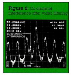
were present 10 kHz from the carrier. (Co-channel interference also can occur at 20 kHz.) Video filtering clears up the display and is very effective for this measurement. Activate the video filter and set it to 30 Hz, and reset the sweep speed to 500 msec/div.
