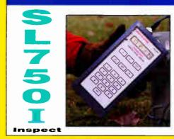
he SL750I was designed to provide you with a quick. accurate, easy-to-use meter that will stand up to the rigors of field service work. The SL750I gives you the ability to test the signal level and HUM on all channels delivered by your system to the customer's home.
