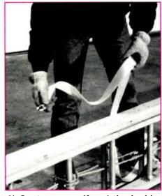
2) Center yourself and the Ladder Tote beside the upright ladder. The adjustable buckle should be on the front end (direction of movement).
