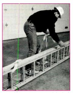
5) Secure the other end of the Ladder Tote to the ladder rail three rungs from the center position in the opposite direction.
