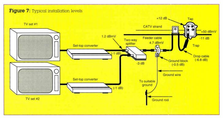
your levels are significantly different than those predicted, then there may be a fault in the installation. To locate this fault we will use the signal level meter to troubleshoot our installation, starting back through the drop.
