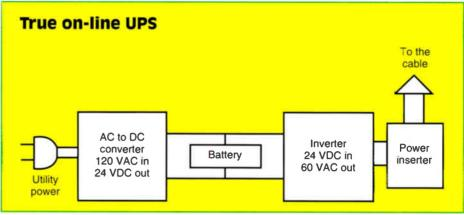
sistors alternately turning on in such a way that they draw current through one-half of the primary of a transformer winding, then switching to the other half so that a square wave is produced on the secondary of the transformer. Various pulse-generating circuits assure that the multivibrator continues to oscillate. These inverters generally operate from 24 VDC.
