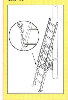
fore climbing and is the most commonly used because it is the quickest and easiest to use. The ITC-6003 has two quick release buckles for rapid setup and take-down. The ITC-6004 (Figure 2) does the same operation as the ITC-6003 except it uses straps around the ladder rail rather than hooks. Key benefits of using the Safe-Tie are:
