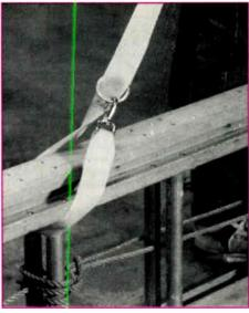
4) The built-in snap and ring secure Ladder Tote to the ladder.
