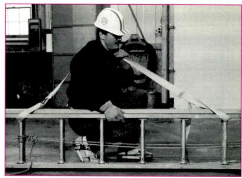
7) Now the tech adjusts the Ladder Tote buckle removing slack until the ladder can be lifted and carried about hip-high.
