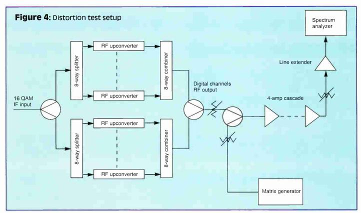
The effect of distortion as a function of digital bandwidth also was verified. This was done by measuring the adjacent channel noise floor with and without the digital signals present as described in the preceding paragraph and calculating the distortion using Equation 11. The number of digital channels was then reduced from 16 to 14 by disconnecting
