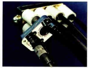
The Freedom Tool shown installing cables in security sleeves
