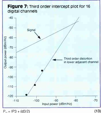
Suppose we wish to maintain a distortion level of -53 dB relative to the digital signal. Then, using Figure 7 and Equation 13, the output power is computed as follows:
