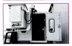
The bucket can be equipped with optional fiberglass lid and full splicing curtain, folding seat and bucket heater. It allows the operator to position the bucket for convenience in cable splic-
