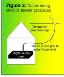
substandard indoor cabling, corrosion, tampering and vibrations all contribute to signal degradation."<sup>2</sup> Digital signals have specific drop level requirements and need consistency in their path:
