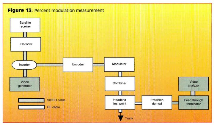
The maximum RF envelope amplitude occurs at the sync tips. The minimum RF envelope occurs at the whitest part of the picture. To properly measure or set the percent mod, the modulated carrier must contain both sync tip peaks and a 100 IRE white signal. If suppressed or stripped sync is used in your scrambling system, the scrambling must be turned off or a procedure permitting measurement of the unsuppressed sync during VBI must be used.
