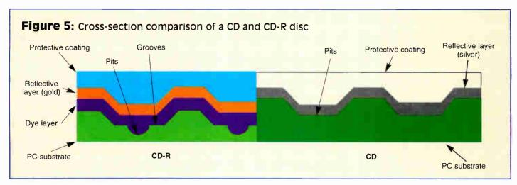
and track width of a CD are almost identical to those of the laser disc. The CD pits have a constant width of 0.5 micron, a depth of 0.1 micron and consist of nine different lengths ranging from 0.86 to 3.18 microns — the track width is 1.6 microns. The recording and playback of a CD is CLV and the track velocity in nominally 1.3 m/sec. A functional diagram of a read-only CD player is shown in Figure 4 (page 22).
