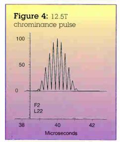
any speed differences encountered because of being at different frequencies become readily visible through predictable distortions of the 12.5T sin² pulse. Generally, the higher chroma frequency will encounter more
