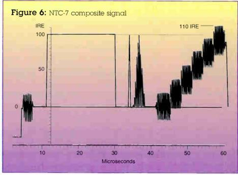
delay than the luminance signal so the test is probably named for this. However, negative delay, where the chroma component arrives first is not uncommon.
