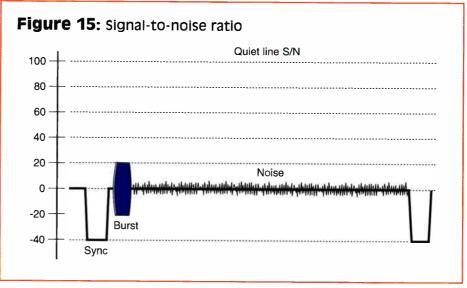
usually the result of poor video source material, an equipment failure, or when very distant off-air signals are brought in via marginal means. While most system sources of noise are flat across the spectrum, noise generated by imaging devices, microwave transmitters and satellite transponders is not flat. Generally, noise increases as the square of the frequency. This is a good reason to insert your own test signals using a VITS insertion generator.
