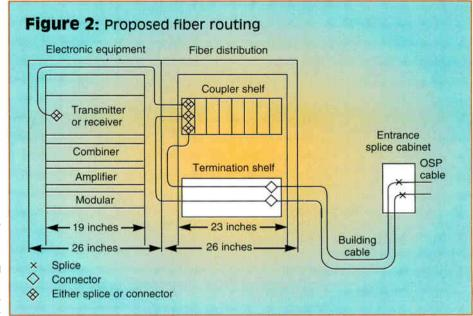
loss performance of splicing was preferred to optical connectors for attaching OSP cables to inside equipment. Early connectors also generated reflectances with magnitudes that caused discomfort because of the widespread uncertainty about their effects on AM systems. The prudent course was to minimize both loss and reflectance by using splices.
