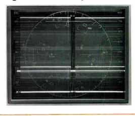
distortions are lower than the hum level you are attempting to measure. Hum distortion will commonly be a sinusoidal distortion at some low frequency (i.e., field or 2X field rate).
