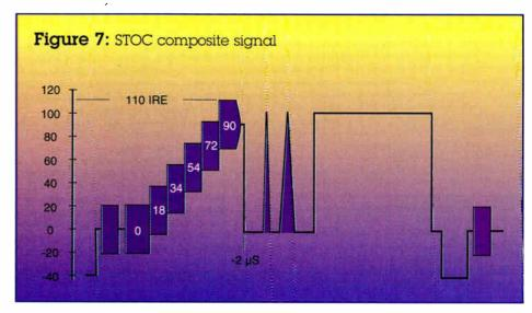
signal and can be easily mistaken for it. The differences, however, between the STOC and FCC composite signals are the chroma peak amplitude in the fifth stairstep, and a 2 µs shift forward in time of the rest of the signal components after the fifth stairstep.
