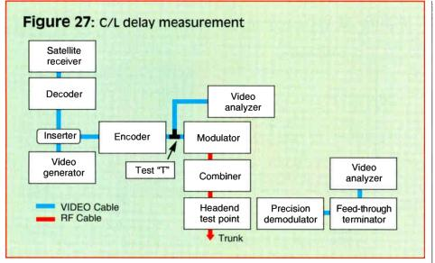
out interrupting the channel. Be sure that only a single 75 ohm termination exists on each video line.
