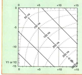
d) Assign the first half of the pulse's base line the variable Y1 and the second half the variable Y2, then apply the chart in Figure 30 to determine the sign for the measurement result.
