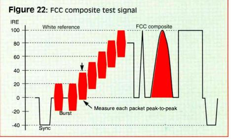
measurements, makes the calculations required for this complex measurement and digitally displays the differential gain on the LCD. The following sections provide detailed information on the FCC Rules and Regulations, a definition of the test, a measurement procedure and many helpful hints and precautions.
