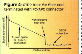
ing percentage than the fiber nearest to the OTDR. In this case the link should be tested from both ends and the loss measurements for this splice be averaged together to find the actual loss of the splice. Additionally, all fiber measurements with an OTDR should be made from both ends of the fiber and averaged together. This provides the most accuracy in length and loss measurements.
