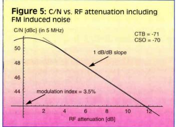
At the distortion levels shown, (CTB = -71, CS0 = -70), the C/No at PAL filter bandwidth of 5 MHz is expected to be 51.4 dBc.
