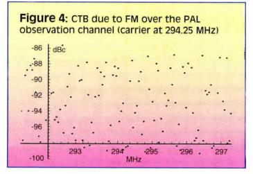
ter bandwidth is shown in Figure 4. Notice that the CTB contribution is scattered in random manner over the entire channel band at a level that is about -85 dBc. A similar noise-like behavior is observed for the CSO contribution of the FM channels.
