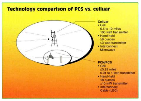
tem that would "find you anywhere," yet employ small, lightweight and inexpensive transceivers - even as compared to cellular. PCS would permit a user to move from small cell to small cell, allowing uninterrupted service from any location. It also would allow, as envisioned by some, connection(s) for home or office equipment such as fax machine, computer, pager, etc., thus possibly even replacing the twisted-pair entry to the home at some point in the distant future.
