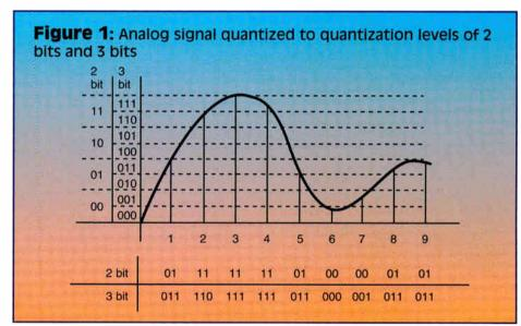
operations are performed in the digital format the resultant digital signal must be converted back into an analog format — digital-to-analog conversion (D/A) — for use in the real world.
