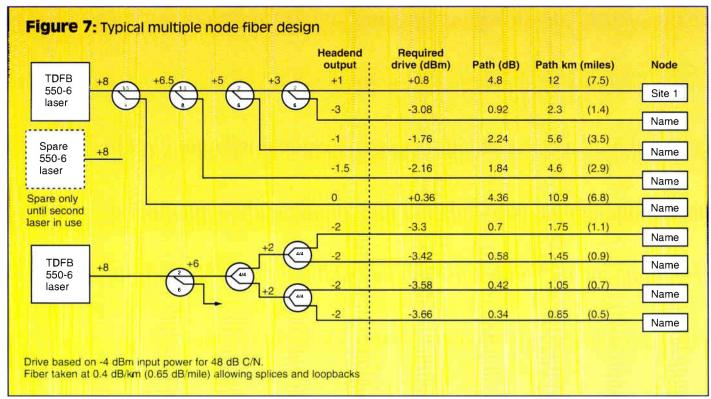
should plan at the outset to lay four to six fibers to each receive location. We can see how even four fibers could be quickly exhausted if we use one for cable, one for return signals, one for digital, and one for the future (a spare).
