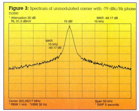
dBc/Hz. Figure 3 shows a typical phase noise plot.
