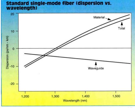
Dispersion-shifted fiber coincides with fiber's low attenuation point, making it suitable for cable TV applications requiring delivery of AM video over long distances and high bit-rate digital applications, such as video-on-demand and two-way interactive multimedia services.
