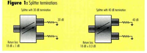
specifications being loosened. For example, the typical 25-30 dB portto-port isolation spec for a highquality 600 MHz splitter has been reduced to 18-25 dB for 1 GHz products. Acceptable return loss (RL) specs also were dropped from a typical range of 22-28 dB to 16-22 dB for similar reasons.
