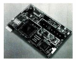
dard board-level QPSK headend receiver provides robust performance in the presence of impulse noise and other channel degradations, while providing the necessary digital signal processing to demodulate signals that have been optimized for upstream transmission over hybrid fiber/coax systems. Prototypes of the unit have been tested using actual upstream echo profile measurements from cable plants. The results showed degradations less than 0.5 dB, according to the company.
