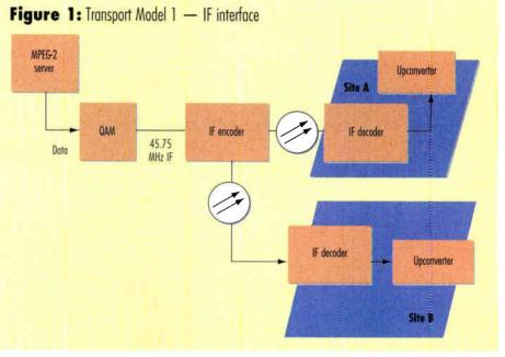
An uncompressed digital backbone offers large networks as great as a 40% advantage in equipment costs over SONET, which requires a codec at each site for each channel. (For scrambled signals, a SONET-based system also must provide a scrambler at each site for each channel.) The uncompressed video transport system requires less equipment and allows all key components such as encoders, scramblers, etc., to be centralized at the headend.
