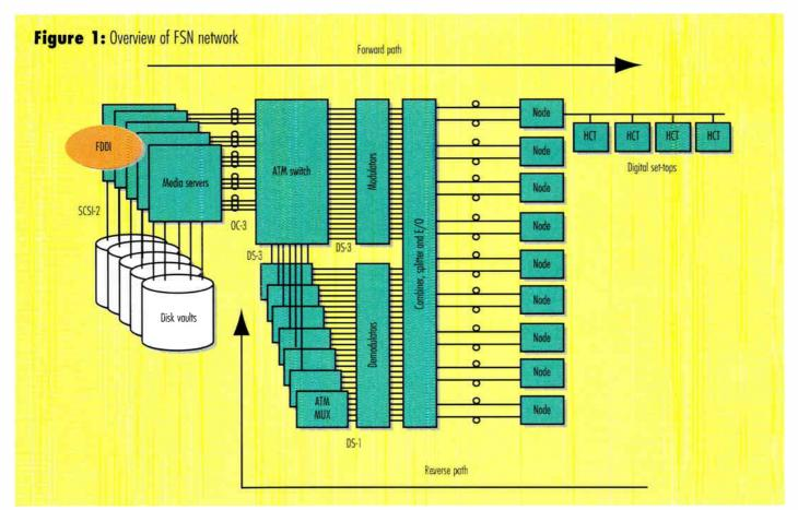
MPEG-compressed video and audio to the subscriber residence. The subscriber is provided with a digital set-top, called an HCT (home communications terminal), which translates the compressed signal back into standard NTSC video and stereo audio. Figure 1 gives an overview of the FSN network. The description is divided into forward (from server to HCT), and reverse (from HCT to server) paths for clarity.
