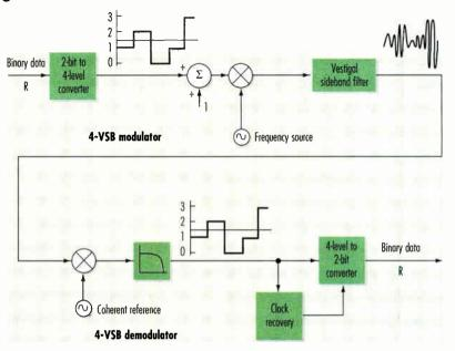
Only one symbol need be transmitted for each pair of data bits, so the symbol rate is half the bit rate.
