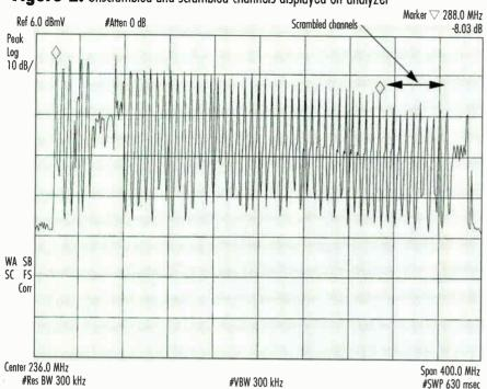
Figure 2: Unscrambled and scrambled channels displayed on analyzer
