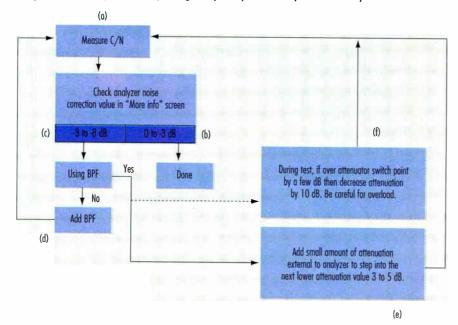
the best, and somewhat hidden feature is the ability of some cable TV analyzers to judge their own accuracy after each measurement. When making a C/N measurement with one such cable TV analyzer, the measurement screen has an information page you can bring up after each test. (See Figures 3 and 4 on pages 62 and 64.) The key to the measurement's accuracy and repeatability is found in the line called "analyzer noise correction." The
