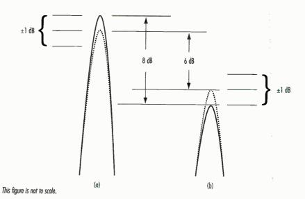
First, check your test equipment specs. They may not be good enough to make the measurement no matter how automatic. The equipment may never be able to make the measurement because it was not designed to provide the level of accuracy you require. In fact, its error may be greater than the tolerance
