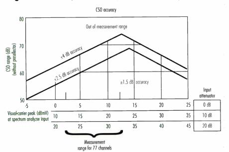
set the attenuator to the highest value at which the distortion signals "track" the attenuation changes, and you will be assured that the CSO/CTB is from your system not the analyzer.
