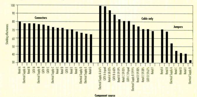
When installed properly, most connectors perform very well. In the case of premade retail jumpers, the damage is already done, with shielding effectiveness dangerously low. The connectors, on the other hand, were installed by well-trained installers using quality cable. The culprit in the case of the jumpers: poor cable-to-connector termination.
