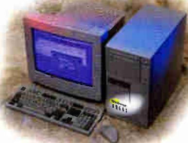
Argus accepts composite, Y/C, YUV, Serial D-1 video and inputs for two analog or digital (AES/EBU) audio channels. It supports closed captioning and uses the Windows 3.51 NT graphical user interface for ease of operation. It's there when you need it...performs at a high level... and applies itself in a variety of roles.
