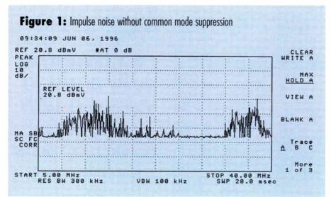
use. As before, a cable-compatible TV set was connected directly to the input of a spectrum analyzer via a length of drop cable. Instrument settings were as shown in the figures, including display max hold to capture as much of the impulse noise as possible. To generate impulse noise, the TV set was turned on and off repetitively.
