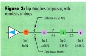
and will have a loss of 4.6 dB at 40 MHz. The equalizers will add about 1 dB insertion loss. Therefore, the actual losses of a 6 dB equalizer will be 1 dB at 750 MHz and 5.6 dB at 40 MHz. Figure 2 considers the previous example again, but this time adds equalizers to the drops; the loss figures are charted in Table 2.
