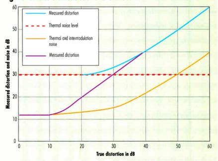
spaced, the distortion products fall in a finite bandwidth. This mandates that a finite bandwidth be used for the measurements. The typical bandwidth used to make this measurement for a cable TV system is 30 KHz.<sup>2</sup> For other situations, such as a cellular telephone amplifier, the products may be much closer together and so allow the use of a narrower resolution bandwidth.
