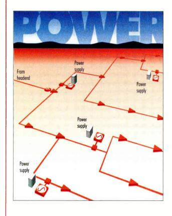
Figure 3: Centralized node powering
