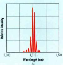
source (the full width at half-maximum designated by  $\Delta\lambda$ ). (Spectral width should be determined for the laser under modulation, since effects like "chirping" can effectively broaden the spectral width.)
