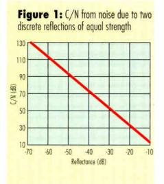
dB, and that reflections of about -30 dB are required to reduce C/N to levels near the cable TV limit of 50 dB. In most cases, if discrete reflections are kept below -40 dB which is the specification for most commercially available splices and connectors—C/N degradation should not be a concern.
