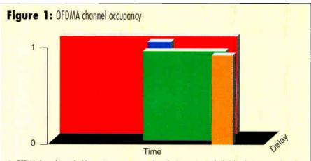
An OFDMA channel is typified by contiguous occupancy along the time axis, at a bulk delay that corresponds to the subscriber's electrical path length. Constant bulk delay "per channel" simplifies upstream dynamic equalization over the entire band.
