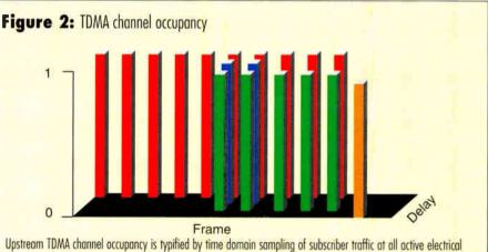
Upstream IDMA channel occupancy is typitied by time domain sampling of subscriber traffic at all active electrical pathelengths. This occurs within a single data frame. Thus, dynamic channel equalization is rendered more difficult. (Note: Sample density not to scale.)
