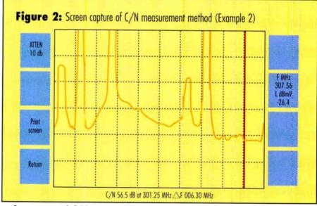
In automated C/N measurement, a signal-to-noise (S/N) measurement is sampled during quiet lines of the vertical interval. With some fancy processing, this results in a C/N measurement. Like the first, this process also is limited because of noise contribution—the sum of the total combined noise sources starting at the broadcast point. (Editor's note: This method will provide an indication of the total noise seen by the subscriber.)
