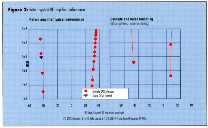
was transmitted through the system. Performance of the system was measured by monitoring the BER as a function of RF level, both through the entire return system and through the fiber link individually. Both F-P and DFB lasers were used separately in the return transmitter to determine the laser's impact on the dynamic range performance of the system.
