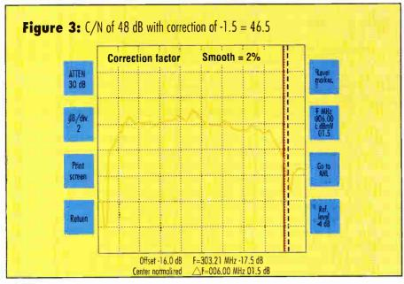
This method is very useful for checking the plant part of the system independently, without including the variable of the previously mentioned methods. When this method is used, you also must check for any roli-off between the two points of measurement. This can easily be done with a sweep system.
