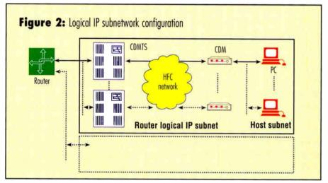
(MAC) protocol and physical transmission medium of the physical layer of the HFC access network. A router provides all internetworking between different customer PCs and the wide area network (WAN).
