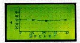
When equipped with the Multiplexer Option, the 9580SST accepts signals from up to 8 separate test points and analyzes sweep & ingress from each individually, returning data to as many as 6 SSR field units (A thru F) connected to it. Announcing the Trilithic 9580 Sweep and Ingress Monitoring System
