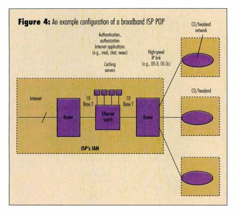
An Internet access subscriber dials up a POTS (analog) or ISDN (digital) connection through the local CO telephony switch to connect to the ISP point of presence (POP), part of the IAN.
