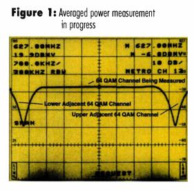
Heavy video filtering is used to average the noise-like signal.
