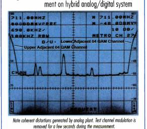
Figure 5: Desired-to-undesired signal ratio measure-
