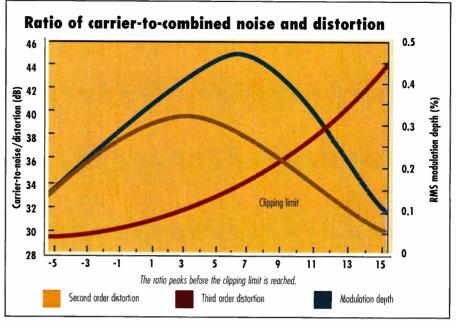
keying (QPSK) or quadrature amplitude modulation (QAM) carriers. A useful way of characterizing the transmission path for these signals is the carrier-to-noise-plus-interference ratio—C/(N+I). This reflects the fact that random noise, harmonic distortion and intermodulation distortion can be combined together to predict the total degradation of the error rates of the demodulated signal.
