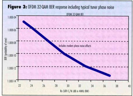
QAM systems with Nyquist filtering can achieve up to N bits/Hz spectral efficiency (with no ingress!), which is the same as OFDM. OFDM is typically generated by a DSP software FFT algorithm. The QAM vector of an OFDM subcarrier is simply set by writing the appropriate amplitude, and phase value into an inverse fast fourier transform (IFFT) frequency bin input. The IFFT transmitter produces a time series signal representation of the summation of all the individual subcarriers from the modem.
