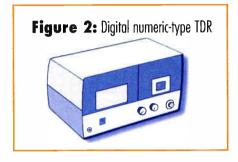
of the cable in order to test. The TDR is "matched" to the cable by entering the velocity of propagation (VOP) of the cable being tested. This enables the operator to obtain the most accurate readings possible.
