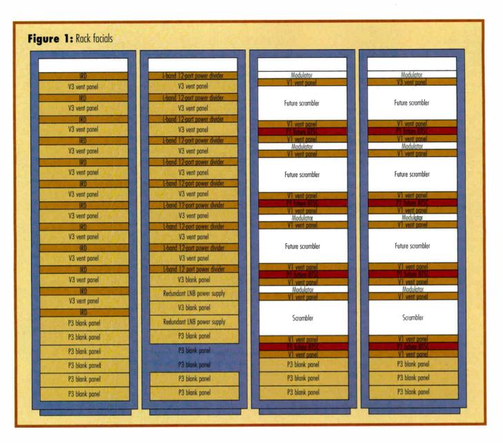
Do some calculations for estimated electrical and air-conditioning requirements. Calculate the UPS size required for the headend racks. Divide the total VA (44,400) by 1,000, to convert to KVA. It is common practice that the UPS be sized 1.5 times the total KVA requirement. (See Table 1 on page 172.)
