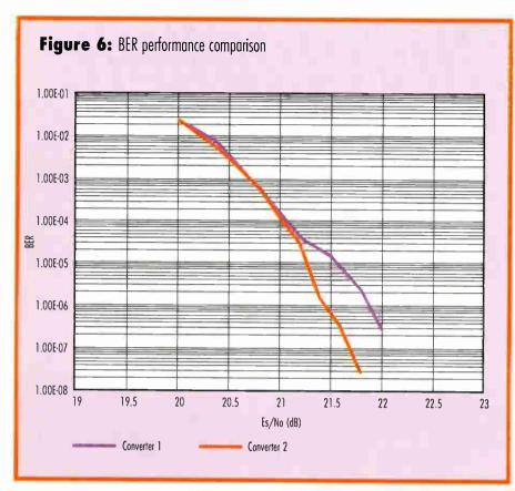
Long-term testing also was performed without introducing AWGN to the system. The test for Converter I ran for 48 hours, 32 minutes with a BER of 6.9E-10. The test for Converter II ran for 15 hours, 36 minutes with zero errors.
