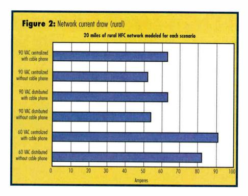
centralized designs. However, by designing with a centralized approach the number of power supply locations was
