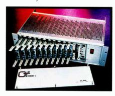
Olson Technology has introduced a compact, modular, frequency agile 12-channel remote control video headend system. The Olson OT-1200 series system features a 5.25- x 19-inch rack-mount housing that contains a power supply and can be configured with any combination of video/audio modulator or demodulator cards. The system operates at frequencies from 54 to 550 MHz and permits local tuning or remote control of each card via a serial data link,
