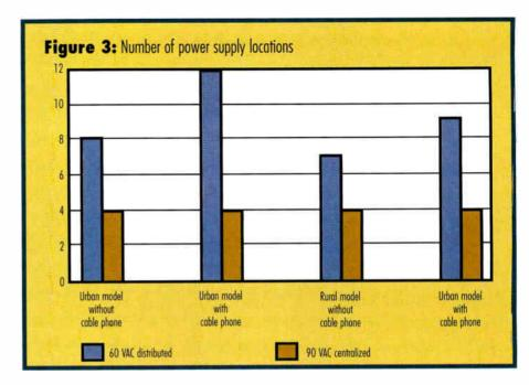
Centralized powering is another way to increase reliability. In centralized powering, power supplies are located at a central point in the system. In most cases, there may be more than one power supply co-located.
