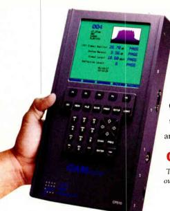
The capabilities of a rack of test equipment reside inside the first truly portable 64 QAM digital transmission analyzer.
