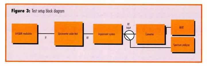
output power was different for both units. These units were off-the-shelf upconverters. Converter I was a fixed-frequency, single-conversion modulator. Converter II was a frequency-agile, dual-conversion upconverter. Both were operated as black boxes with the output level adjusted for maximum output power. Both test unit outputs were attenuated to deliver an RF signal of 0 dBmV at the downconverter's input.
