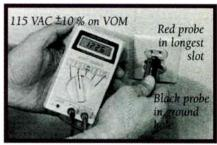
Figure 2: VOM (digital multimeter) indicating improper wiring polarity
