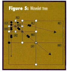
wavelet coefficients are represented by a structure known as a wavelet tree, in which the nodes of the tree correspond one-to-one with the wavelet coefficients. The coefficient at the coarse scale is called a parent, and all coefficients at the same spatial location and of similar orientation at the next finer scale are that parent's children. Figure 5 shows such a wavelet tree with three levels of decomposition.
