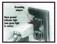
Figure 1: Reading "open ground" indication on AC outlet tester
