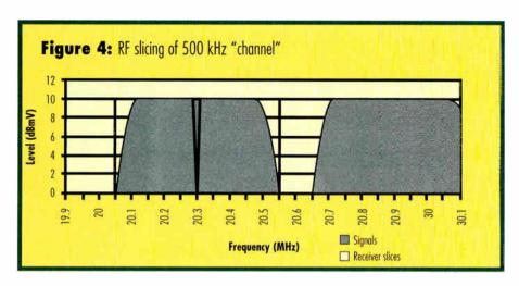
measured are at 600 kHz spacing with 50 kHz internal guardbands on each side, and the RF "slices" are 250 kHz each. If the meter is programmed with a 600 kHz channel centered at 20.3 MHz, it needs to take three slices to cover the band completely, and measures a total bandwidth of 750 kHz. If there is a guardband next to the signal to be measured, this is OK, but extra power may be measured if another signal is in the
