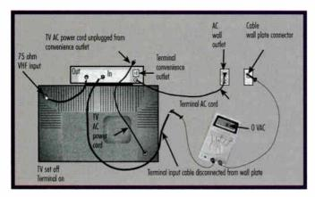
Figure 2: No AC voltage between input cable F-connector nut and F-81 barrel connector threads indicates hot chassis condition at TV set
