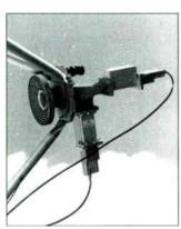
Photo of 7892's mounted between antenna feed and LNA's (both Vertical and Horizontal Polarization).
