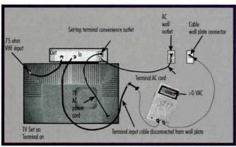
Figure 1: Presence of AC voltage between input cable F-connector nut and F-81 barrel connector threads indicates hot chassis condition at either TV set or set-top terminal
