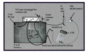
Figure 3: Presence of AC voltage between F-81 barrel connector threads and input cable F-connector nut indicates hot chassis condition at set-top terminal
