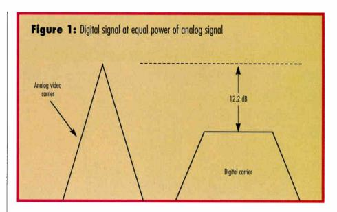
digital installations. When viewed on a spectrum analyzer, the digital signal's energy may appear to be spread uniformly over the entire signal bandwidth, depending on the type of digitally modulated carrier. Conversely, an analog signal has most of its energy concentrated around the visual carrier. The resolution bandwidth of the meter or spectrum analyzer captures all of the analog signal's energy, so no correction is needed. But because the digital
