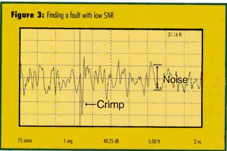
"bumps" on the trace represent real faults, not just noise. Events that were difficult or impossible to find using old generation TDRs with higher SNR (see Figure 3) are visible above the noise because the noise is much lower. This also means that you can clearly see faults further away than you could in the past (see Figure 4).
