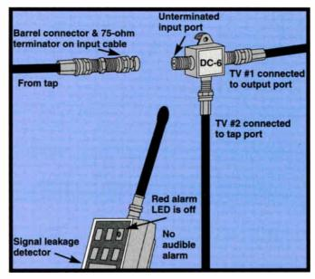
Figure 2: No cable signal leakage present with F-connector on input cable to directional coupler terminated indicates defective directional coupler.
