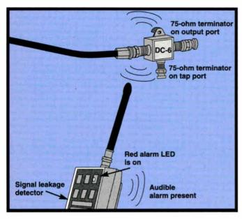
Figure 1: Signal leakage present with output/tap ports terminated indicates defective input F-connector, poor housing shielding or upstream leakage.
