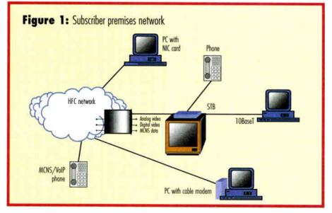
The access network is designed such that the subscriber's equipment cost is the minimum required to deliver the network services. Equipment in the access network includes RF modulators, HFC lasers and fiber, fiber nodes, and RF amps. Ad insertion can be done either in the headend or in the hub, or potentially at the client device with HTML.
