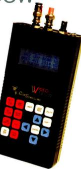
Also does transmission, vectorscope, waveform monitor, camera matching, A-B Tests and sync analysis tests.
