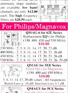
0// 100 C Variable EQ's for Magnavox (330 and 450 MHz) \$14.00 5, 8, 11, 14, 17, 20, 23 dB Values Return Loss  $\geq$  -16 dB. Insertion Loss  $\approx$  1 dB Use our QMAG-P for 4-A Pads
