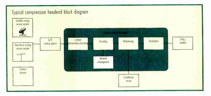
to the digital compression system. At the encoder, the source programs are compressed into a Moving Pictures Experts Group (MPEG) transport stream.
